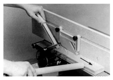
Handle cross grain cuts by working with the miter gauge and using the miter gauge stop rod to determine the depth of cut (Figure 10-19). There will be some feathering at the end of the cut, so work on a piece that is wider than you need. Remove the chip by making a light jointer cut or by sawing.
