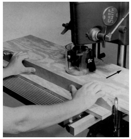
**Figure 10-15**. A sliding table greatly simplifies cutting a dovetail slot in an extrawide piece.
