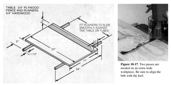
**Figure 10-16**. Construction details of the sliding table. Runners should fit snugly against the edges of the table (Model 500) or the table tubes (Model 510).
